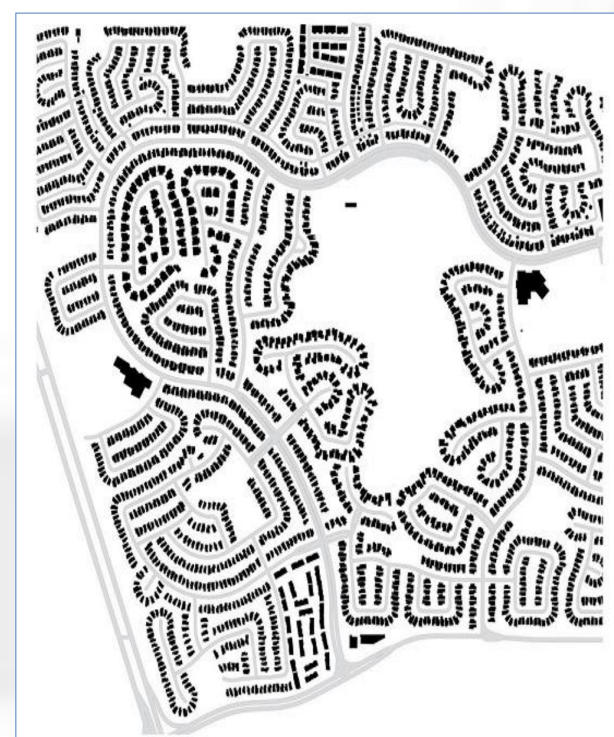
Fig. 1 – A typical Calgary curvilinear street pattern (lines represent roads and polygons represent building)
