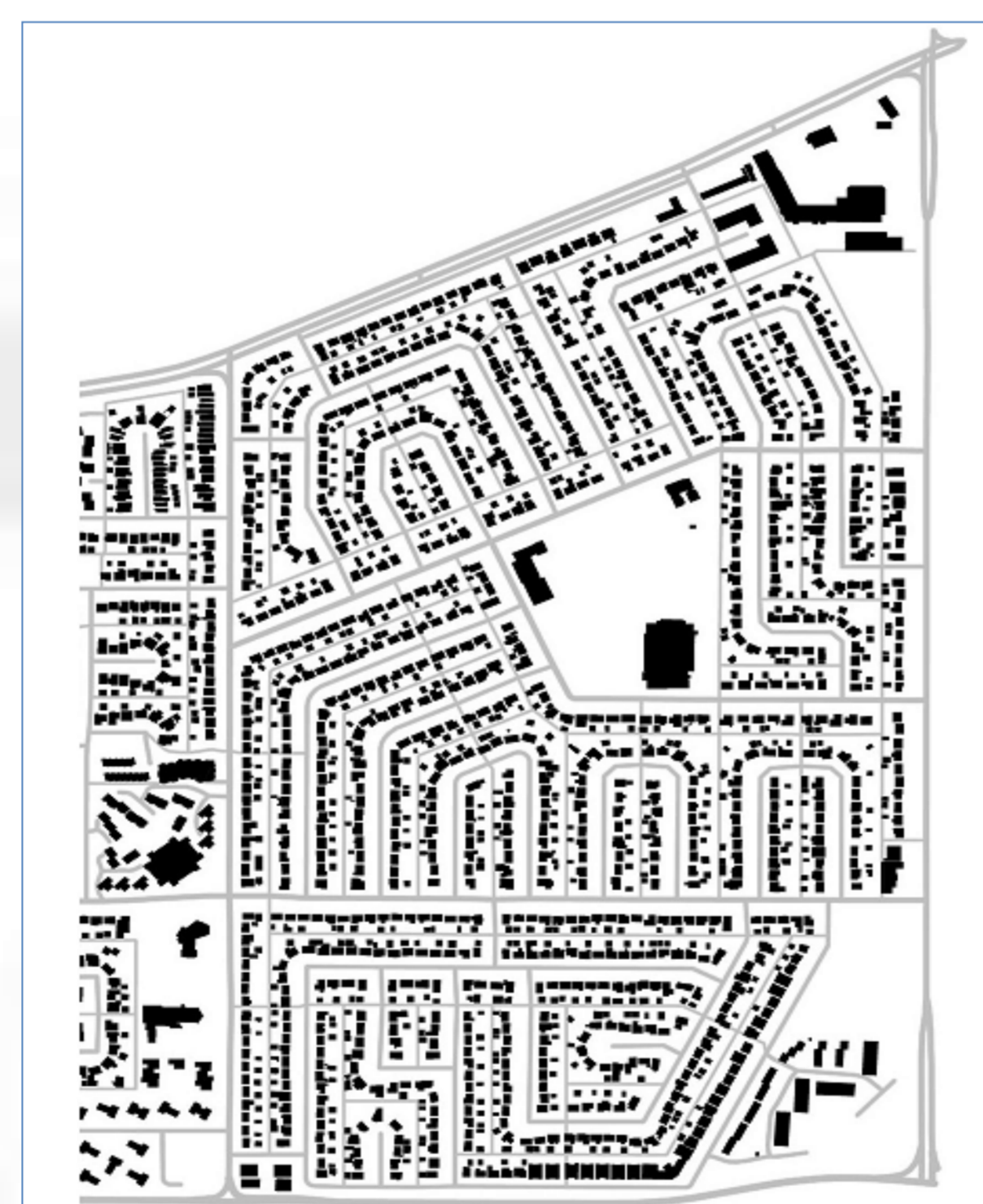
Fig. 2 – A typical Calgary warped-grid street pattern (lines represent roads and polygons represent building)
